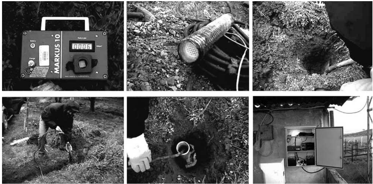
Figure 3. Soil Radon Site selection and deployment of continuously recording radon sensor and establishment of data recording and transfer unit.
