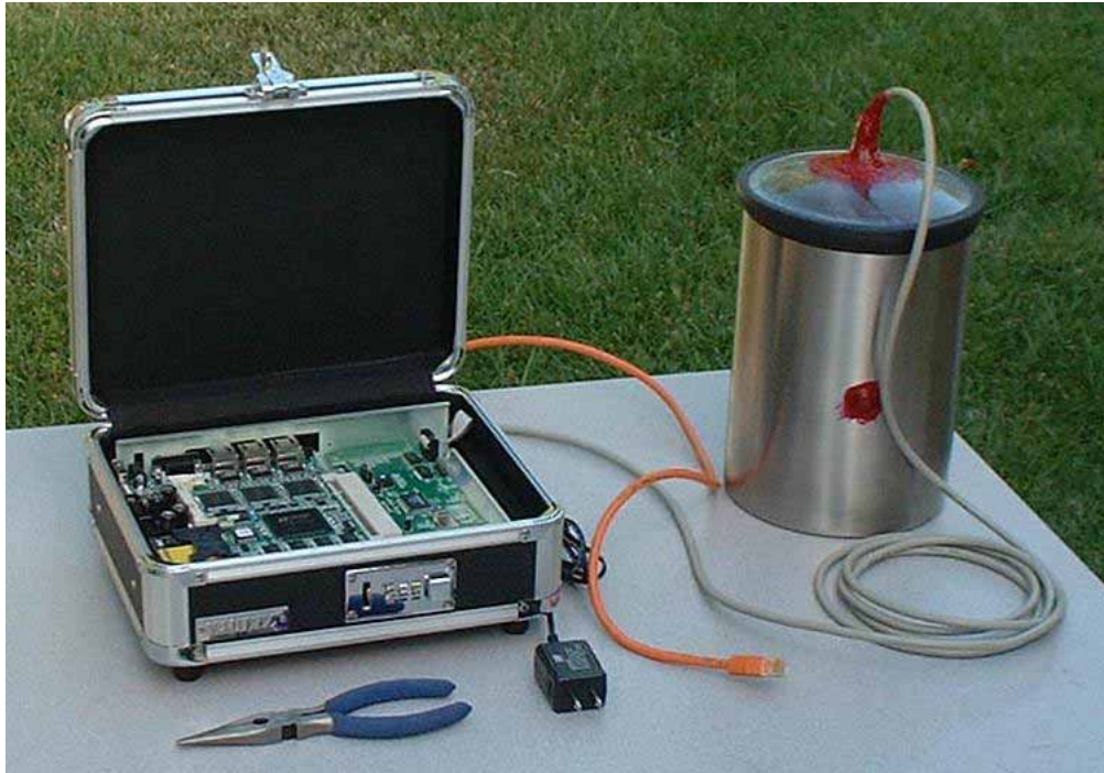
Above sensor system measures displacement as little as 1 nm.
